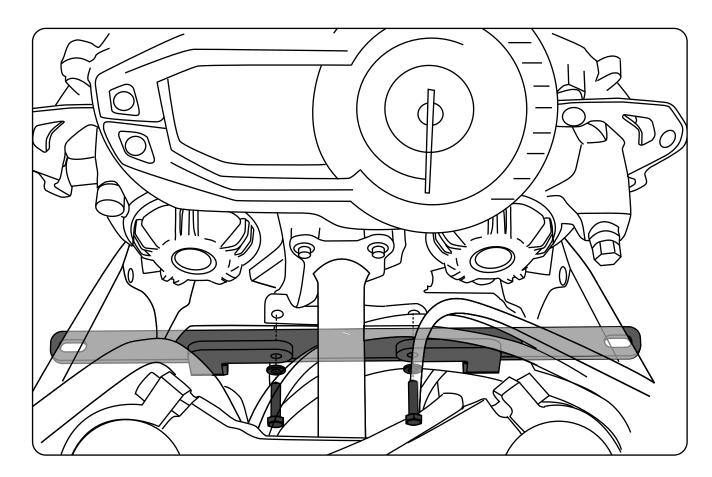
**Step One:** Remove the two lower bolts from the fiaring stay.
