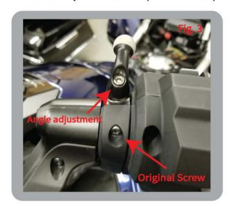
5. Adjust the angle of the ball mount using the allen head screw indicated in figure 3. Once you are satisfied with the angle, tighted it down and attach your desired accessory.
