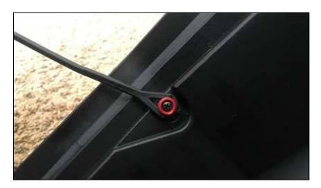
2) Remove the twelve (12) screws along the perimeter of the inside of the case lid. The four (4) screws in the middle must also be removed.
