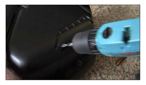
This will allow the wires from the LED array to be routed inside the case.
