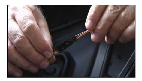
3) Route the excess cables inside the case using the included cable clamps. This will allow the cables to be out of the way while you are using the case. Clean the surface with alcohol before placing the clamps to promote maximum adhesion.
