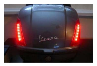
$^{\star}$  Standard kit shown. Premium (CG) kit has 2 LED arrays per side for a total of 24 LEDs per side.
