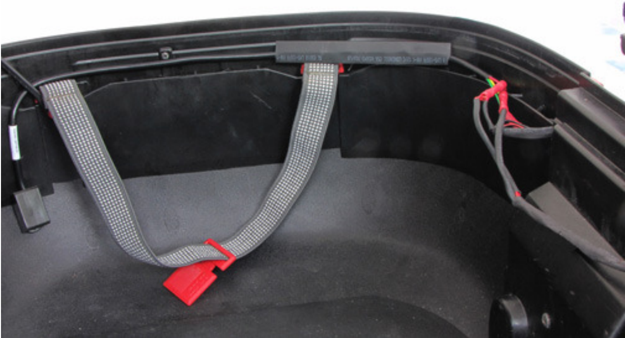
Figure 10: Shrink tubing (before shrinking) slid to the side while couplings are connected.
