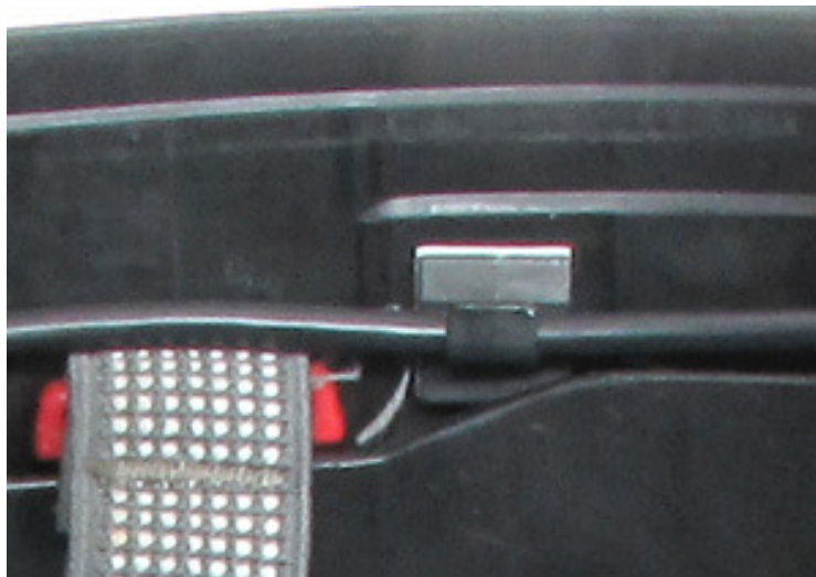
Figure 11: Adhesive cable clamps to secure the wire harness.
