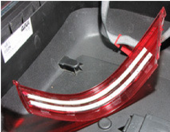
Figure 2: LED Strips positioned in the lens.
