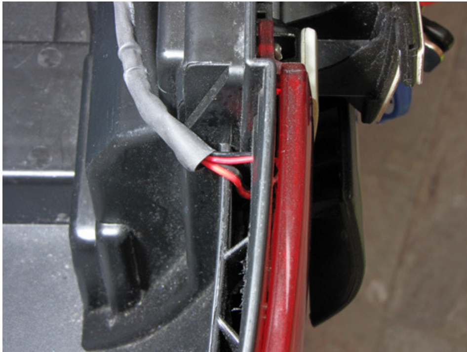
Figure 6: Wires passed through the holes drilled in step ④. Note: Shrink tubing covering the wires is for a later step.
