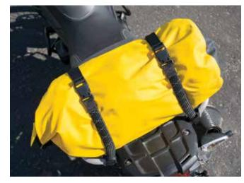
It's easy to use: Undo the plastic side-release connector and simply feed the strap through the loop at each end to secure it to any mounting point of your motorcycle. Reconnect the side-release connector and pull the loose end of the strap to cinch down your cargo.
